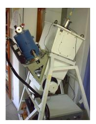
The echelle spectrograph delivered by REOSC (France), was designed to work at the F/15 cassegrain focus of the 91-cm telescope. The spectrograph is designed to work at high resolution, in cross-dispersion mode and at low resolution, in single dispersion mode. Since 1993 the spectrograph is fed by a fiber link and placed in a gravity independent position at the
