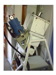
The echelle spectrograph delivered by REOSC (France), was designed to work at the F/15 cassegrain focus of the 91-cm telescope. The spectrograph is designed to work at high resolution, in cross-dispersion mode and at low resolution, in single dispersion mode. Since 1993 the spectrograph is fed by a fiber link and placed in a gravity independent position at the
